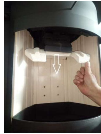
3. Drop and remove concrete deflector.
